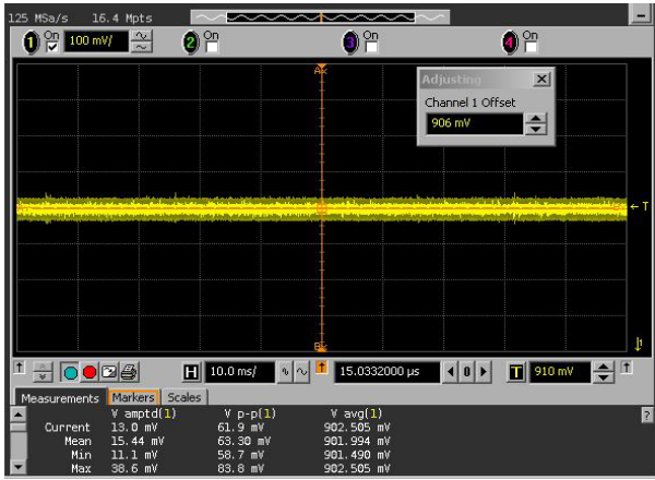
Figure 10: V_{OUT} measured in infinite persistence while adjusting the current drawn.
